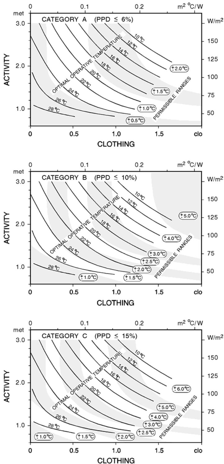
**Figure 1: The optimum operative temperature as a function of clothing and activity for the three categories of the thermal environment. The three diagrams show also the range around the optimum temperature for the three categories.**
